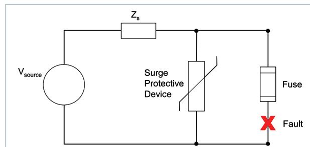
Figure 4. Circuit for transient voltage.
