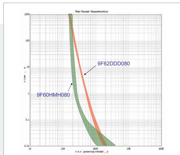
Figure 5. Time current curves for two different 15.5kV 80E fuses.
