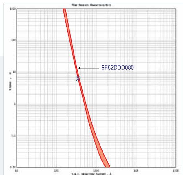
Figure 2: Time current curve for primary fuse.
